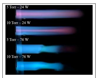
**Fig. 1**. Plasma pictures for four experimental conditions with the bi-colored and diffusive regime.
